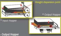
When a card is put in the output hopper, to protect the card's surface, the loaded cards are raised by the support beam which is operated by the internal CAM.
