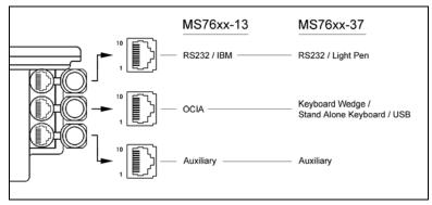
Figure 33: Scanner Interface Ports
