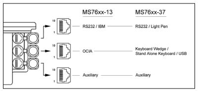
Figure 32: Scanner Interface Ports
