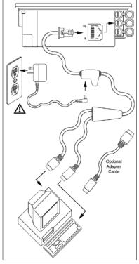
Figure 15: Keyboard Wedge Interfaces
