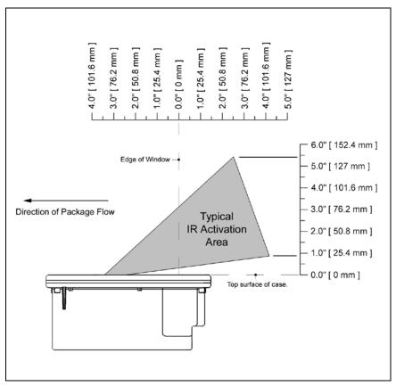
Figure 28: IR Activation Area Parallel to Package Flow
