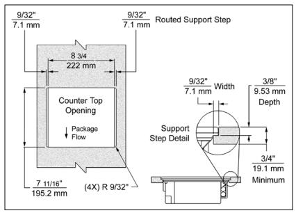
Figure 11: Specifications for Free Hanging Support
