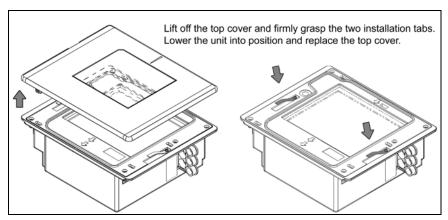
Figure 9: Installation Tabs
