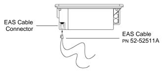
Figure 24: EAS Cable and Connector
