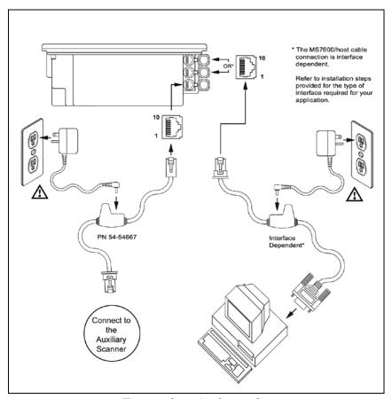
Figure 23: Secondary Scanner Setup
