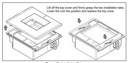
Figure 12: Installation Tabs
